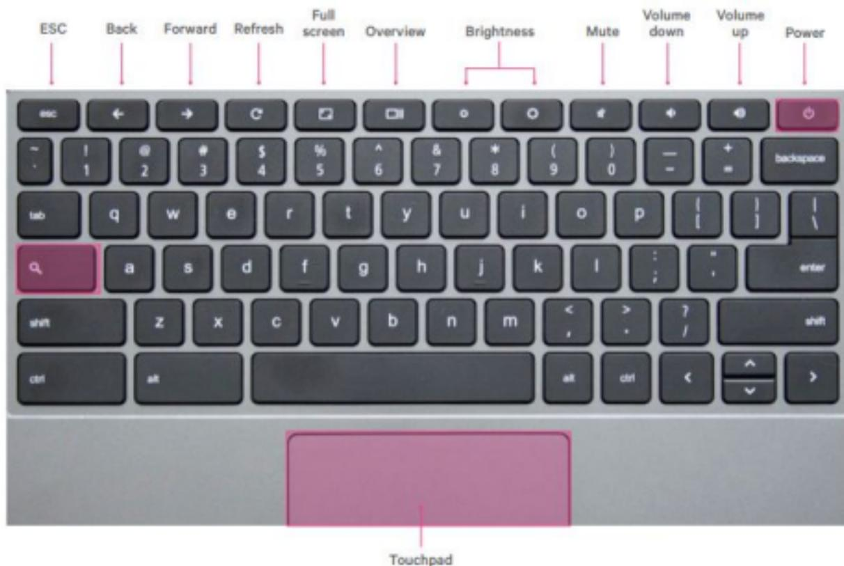
On some models, the Power key is a Lock key. This key locks the computer and will require you to log back on. Look for the power button on the left or right edge of the base.
